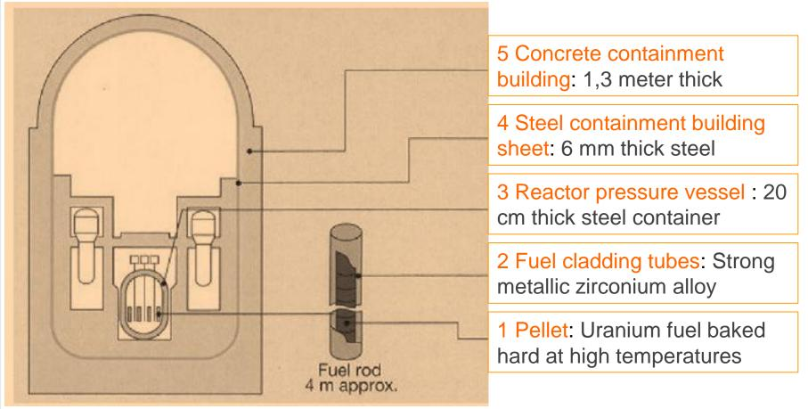
Preventing release of radioactive material
