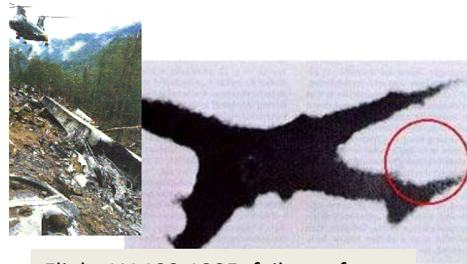
Flight JAL123 1985, failure of design of critical structural repair, not post inspected as required.
