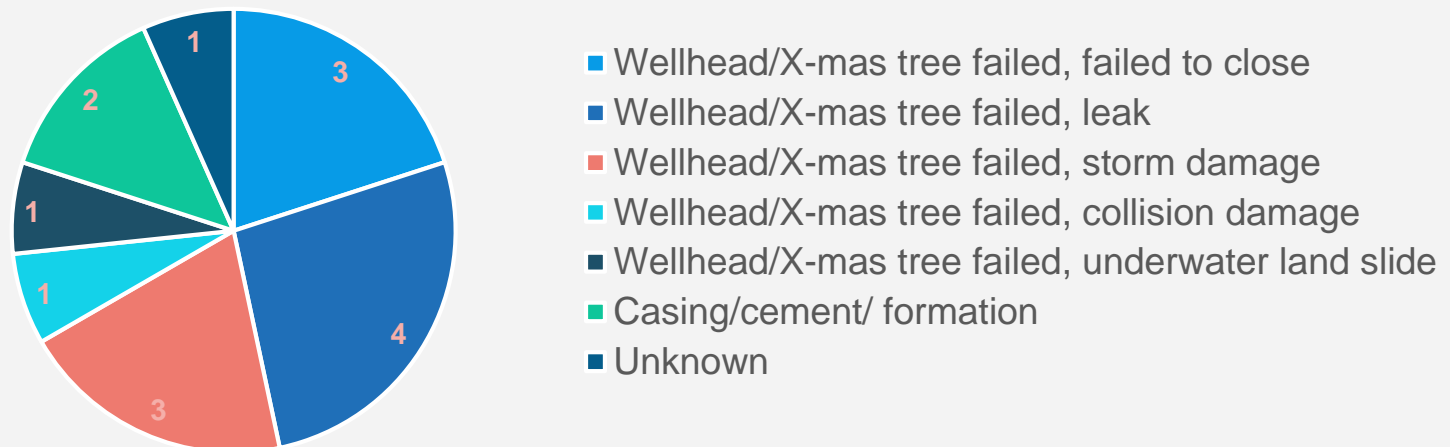
Loss of secondary barrier for production LOWCs
