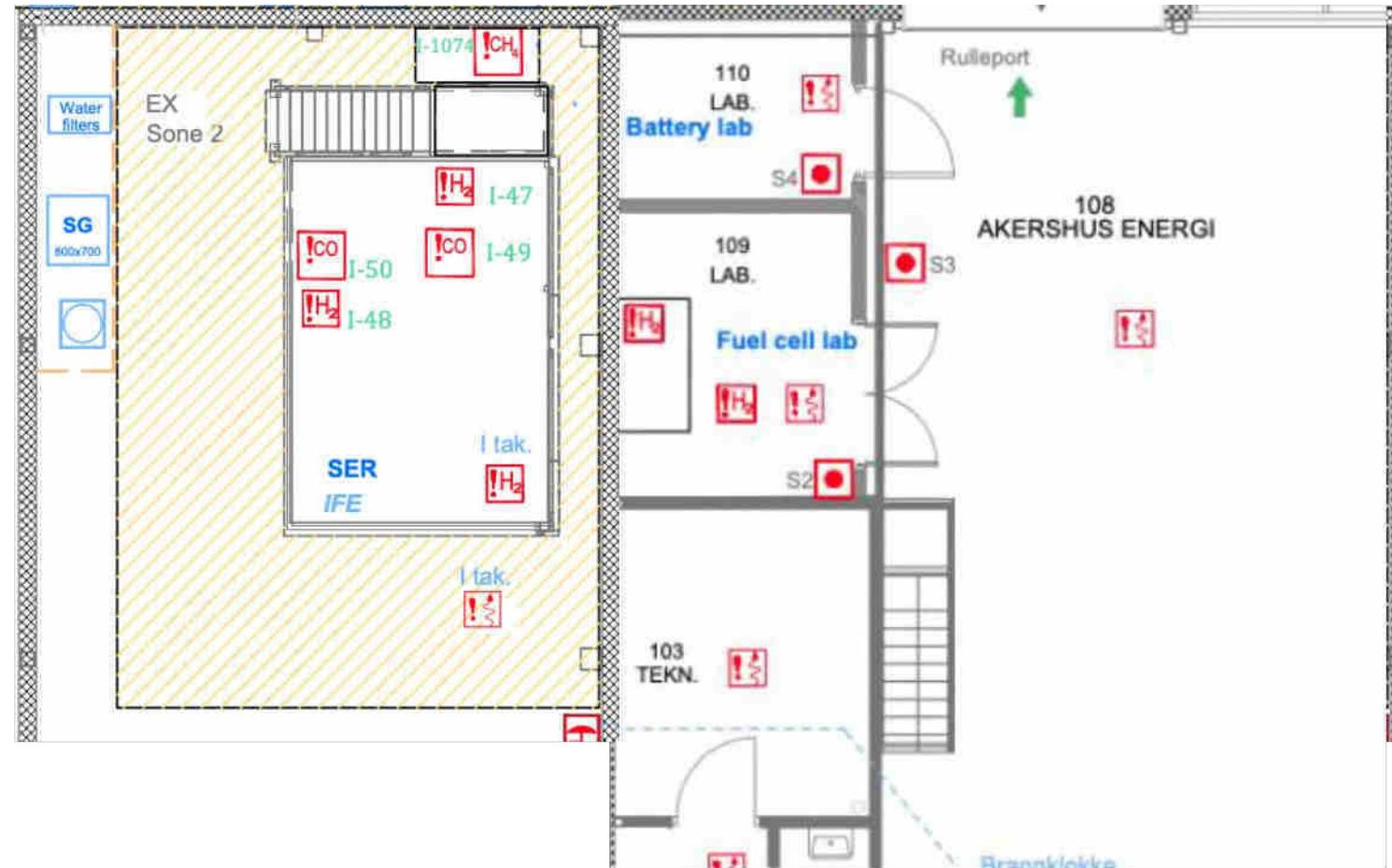
**ATEX ZONE 2** – Hazardous area classified as an atmosphere where a mixture of air and flammable substances in the form of gas, vapor or mist is **not likely** to occur in normal operation, but if it does occur it will **only last for a short period** – **Medium Risk gas/vapor**
