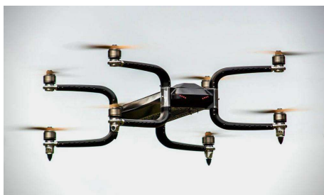
Griff Aviation 300 (Norsk design) ~ 230 kg payload
